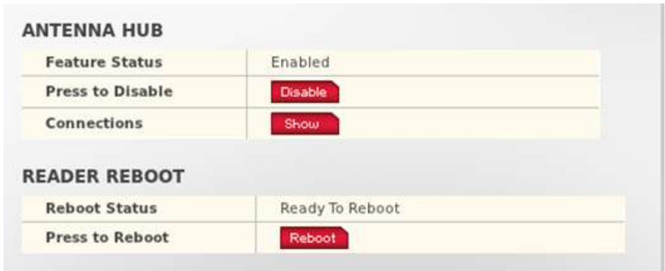
Figure D.2 Close-up of Antenna Hub Section of Reader Management Web Page
