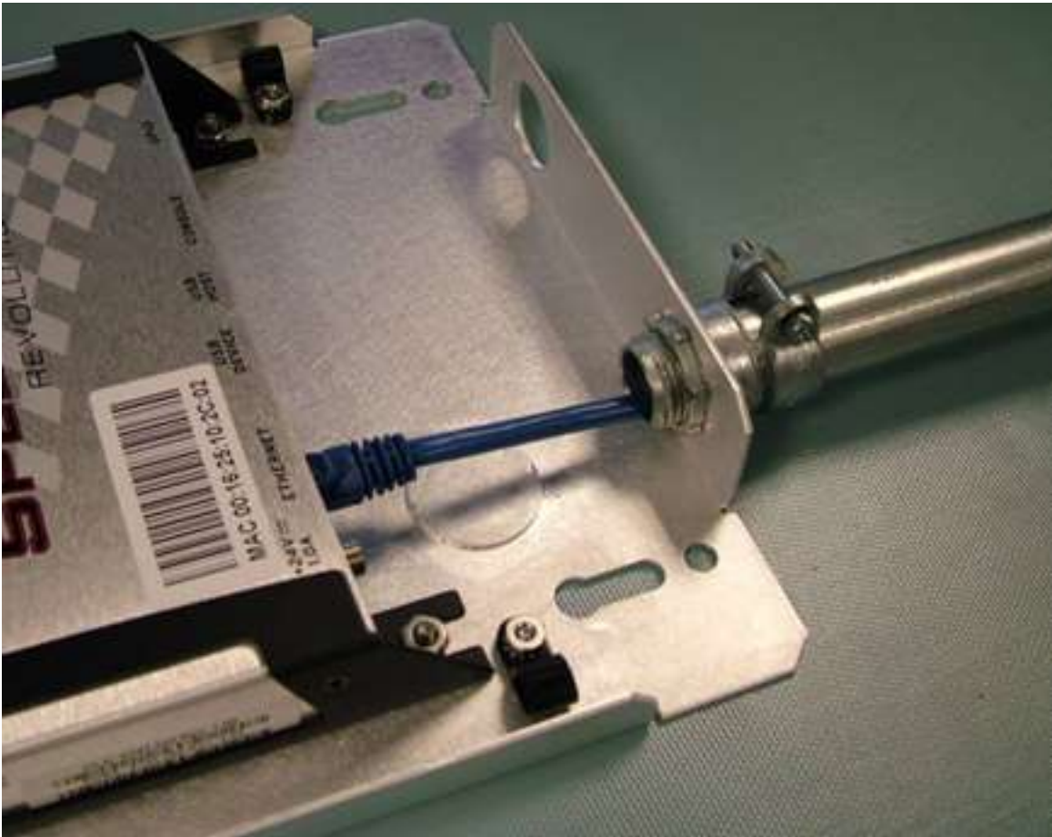
Figure C.7 A squeeze connector for the larger \frac{3}{4} inch conduit tubing size. The connector has a nut and threads sized for the \frac{1}{2} inch conduit hole.
