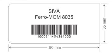
SIVA's Ferro-MOM 8035 is a passive RAIN (UHF) RFID label optimized for Metal and Plastic among other surfaces and delivered with a high performance acrylic adhesive. These labels feature a film face to print customized logos, product information, scannable barcodes, QR codes, etc. directly on the label.
