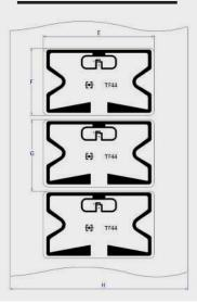
53 mm E- Label Width F- Label Length 32 mm G- Label Pitch 34 mm H- Web Width 85 mm
